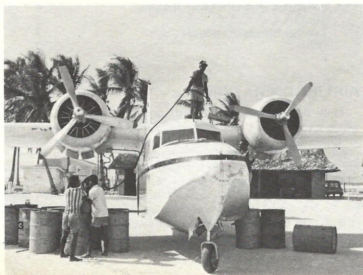
6. Fuller Brush Company's N2943 (J6) is shown in a 1946 photo. Note the sawhorse used prior to installation of the "squat strut." Leading edge slot is also evident in photo. Propeller warning stripe is unusual on Mallards. Peter M. Bowers
