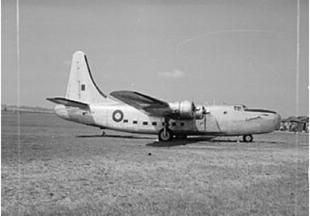
Churchill's Liberator II Commando after modifications were made to its nose and fin.
