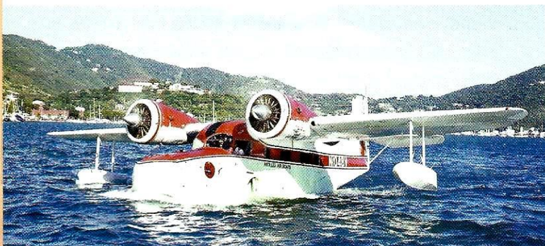
The wheels have already been extended as this Goose is about to engage the ramp leading to the terminal building at St Thomas. These airplanes were powered by two 450hp (335kW) Pratt & Whitney R-985 engines.
