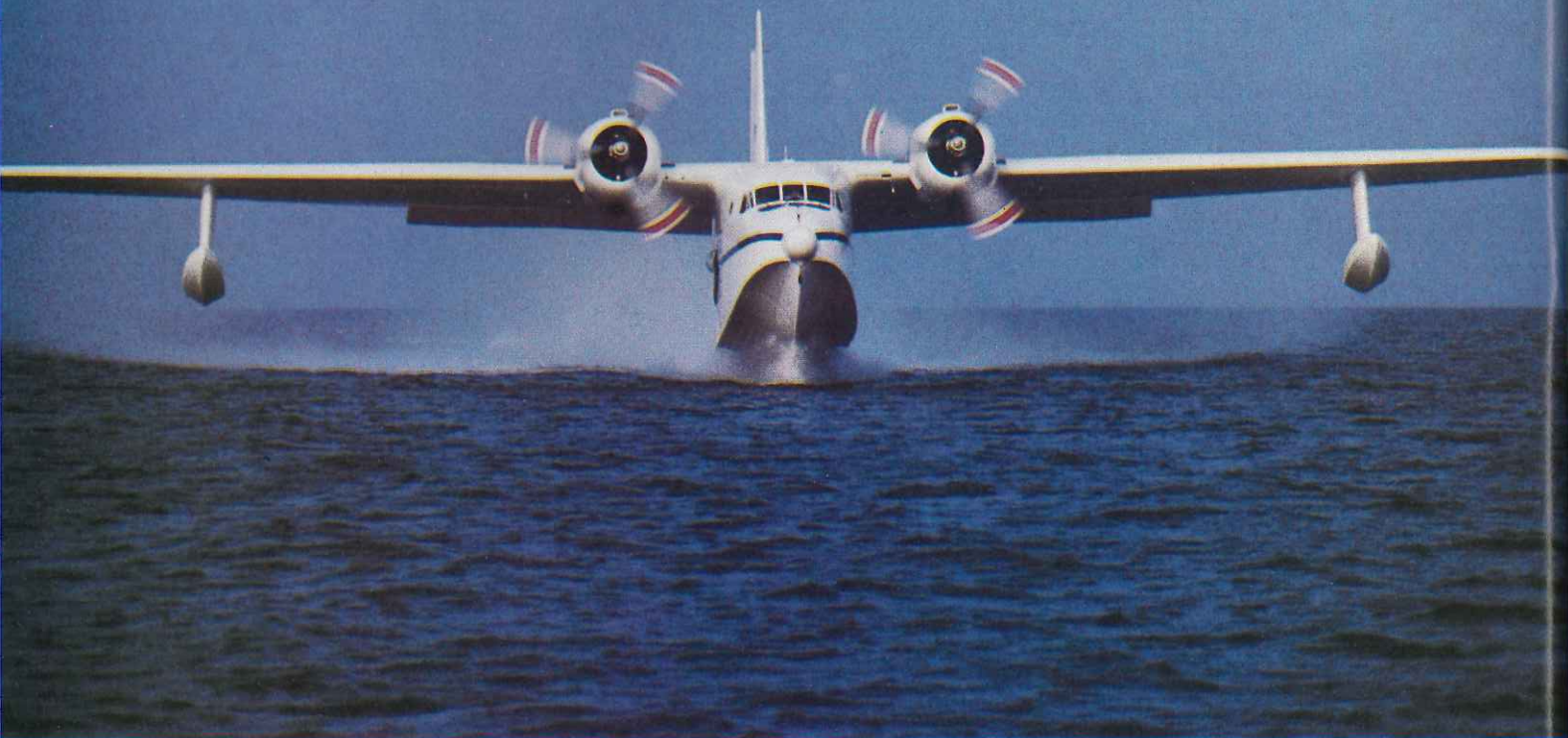
Its two Curtiss Wright R1820-83 radials developing almost 1500 hp for takeoff, prototype G111 Albatross leaves a rainstorm of spray in its wake during performance trials last year. If business warrants, both Chalk's and Antilles might be adding G111's to their fleets in 1981.
