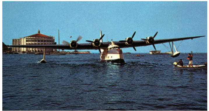
881 approaches with the copilot in the forward hatch waiting to take the pivot line from the dock boy. Note that the right-outboard engine is the only power being applied. (Photo from a scanned postcard from the author's collection).
