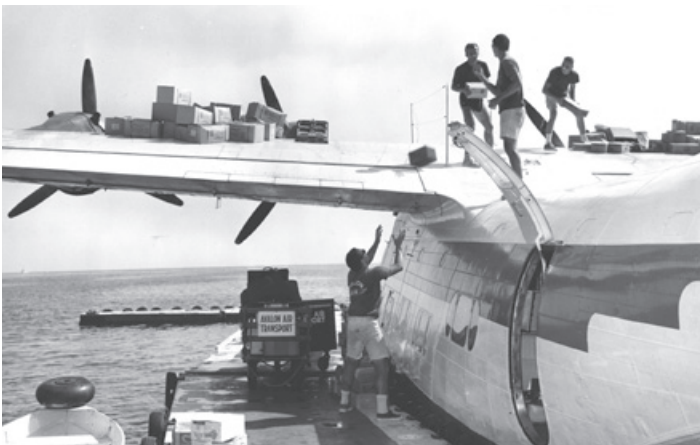
Freight day was a real work out for the dock crews at both the Long Beach Harbor and Avalon seaplane bases. Here, freight is being pulled from the eight wing bins. The author is on the dock about to catch a box of frozen orange juice while David Turner, Joe Waldman, and Tom Flood toss boxes that they will deliver around the town (Photo by a visiting former Pan Am employee - from the author's collection).
