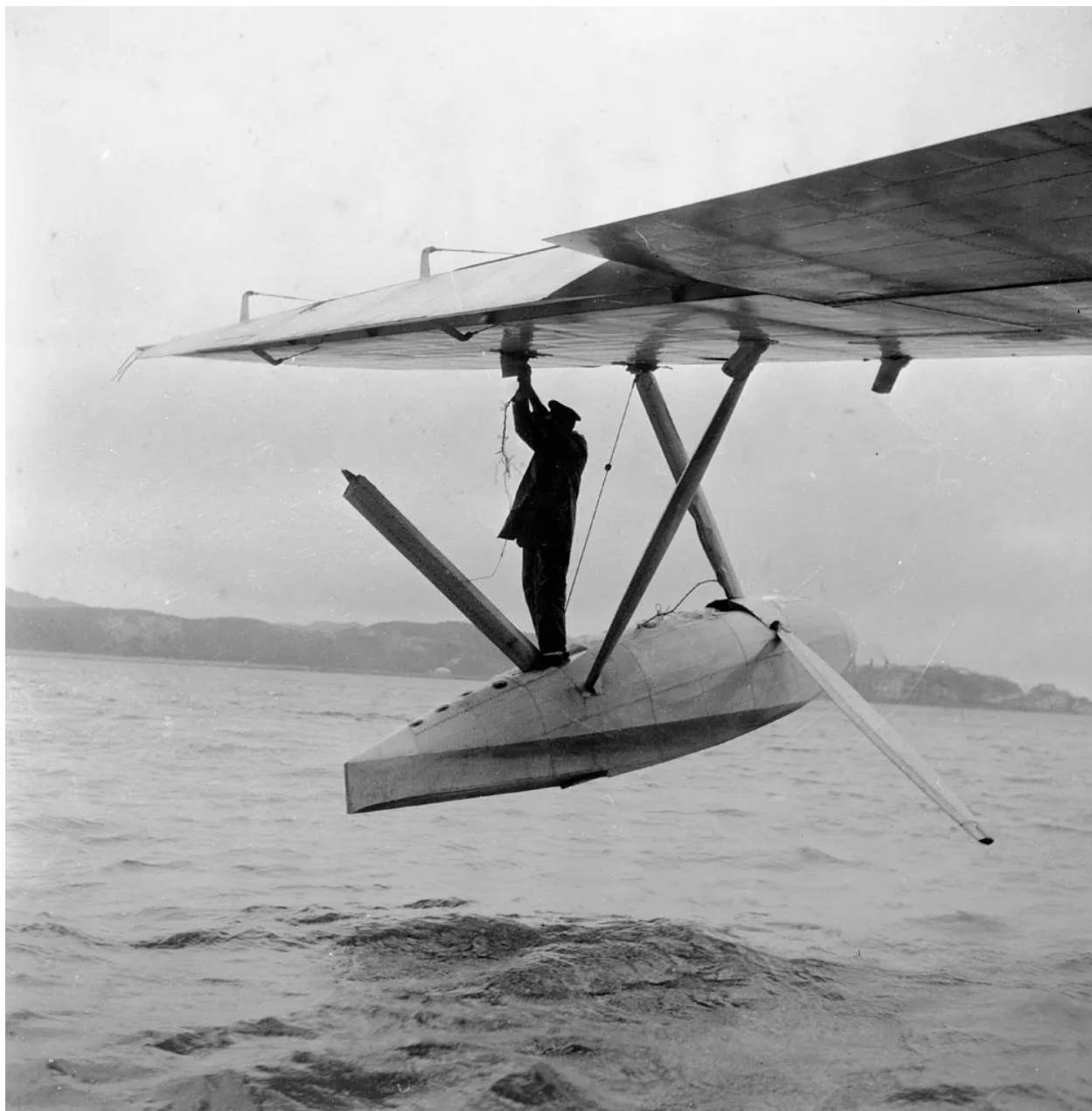
The struts supporting the float were designed to easily detach from the wing without causing further damage. Repairs would take no more than three hours.
