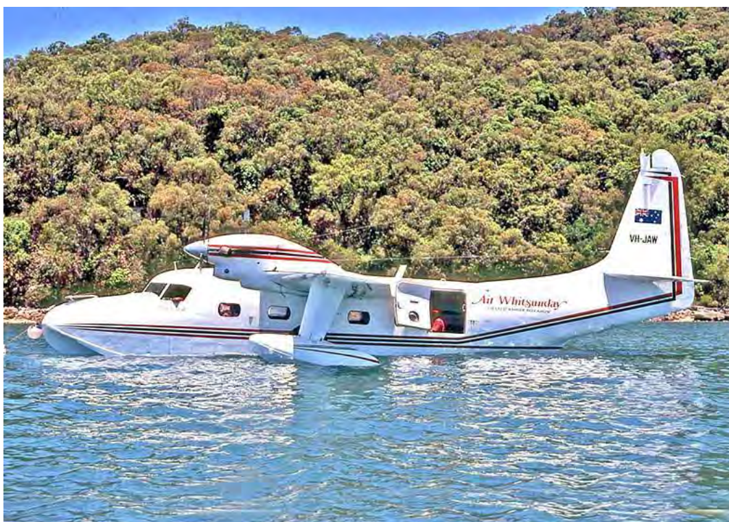
VH-JAW (c/n J-26) also with Air Whitsunday, illustrates the PT-6 turbine-powered Frakes G-73T Turbo Mallard .
