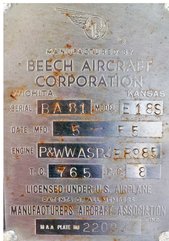
Typical Beech construction plate: BA-81 N3781B, VH-CIJ. (courtesy Ron Cuskelly)
