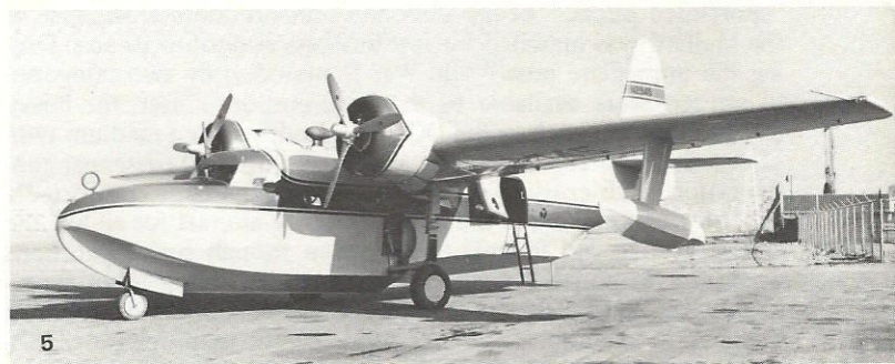
6. Fuller Brush Company's N2943 (J6) is shown in a 1946 photo. Note the sawhorse used prior to installation of the "squat strut." Leading edge slot is also evident in photo. Propeller warning stripe is unusual on Mallards. Peter M. Bowers
