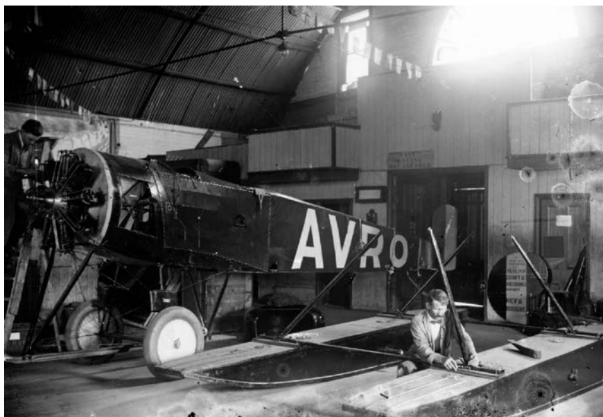
Avro 504K being assembled at the Mascot Australian Aircraft and Engineering Company. Date and origin unknown – Image from glass negative provided by David Vincent.
