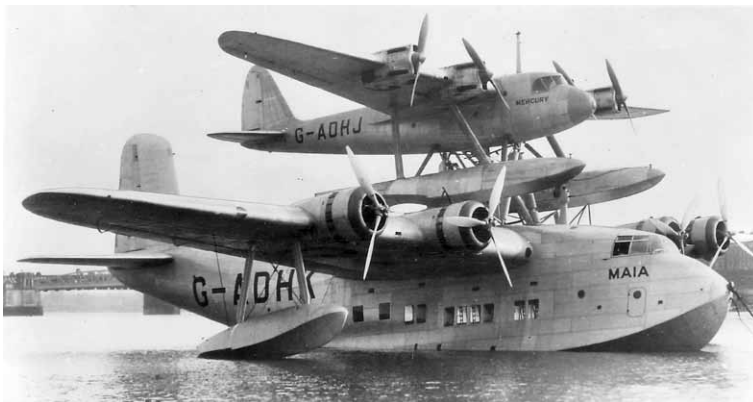
The composite Short-Mayo composite design with the Short S.21, Maia, G-ADHK, mother ship and the Short S.20, Mercury, G-ADHJ, mounted together. (Photo from the Gerald Balzer collection, AAHS archives)
