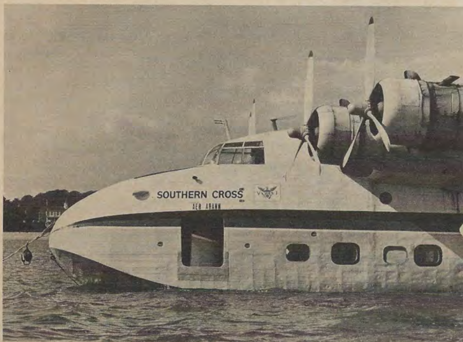
A close-up view of the Sandringham at anchor off Calshot. Note the well-used appearance of the aircraft's skin. Also note how close the entrance door is to the water. The insignia is that of the Virgin Islands.
