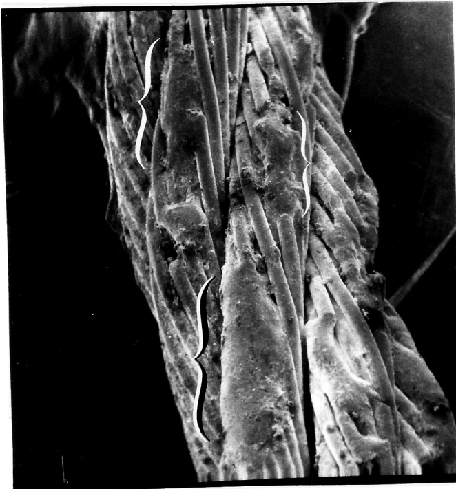
Figure 4. An SEM macrograph (10X) of fused wires (brackets) on the surface of the left aileron cable.
