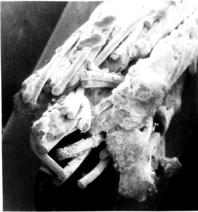
Figure 3. An SEM macrograph (10X) of the fused end of the left aileron cable outboard segment.
