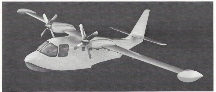
Grumman Aerospace Design 711 started wind tunnel testing recently with a ½-scale model to examine the lift, drag and moment characteristics of the baseline configuration. The 10-place amphibian is designed to incorporate either piston or turboprop engines.
