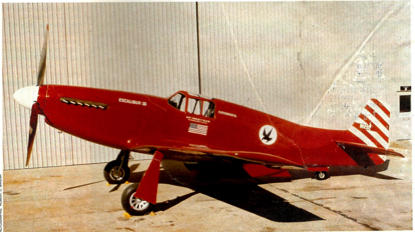
TOP: Blair runs up his Rolls Royce Merlin engine at Bardufoss. The North American P-51C Mustang used for the polar flight was modified in that it had a wet wing, able to hold 690 gallons, supplementing the fuselage tank. ABOVE: Excalibur III after being restored to correct the excessive corrosion of the wings from fuel seepage, ready for display at the National Air and Space Museum, Washington, D.C.
