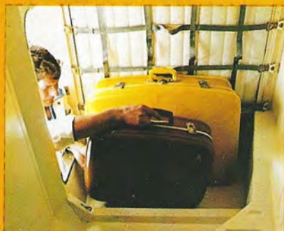
30 cubic feet (0.85 cu. m) rear baggage locker. Standard on N24A — optional on N22B. Carries 200 lb (91 kg). Door size 21"x29" (0.50 m x 0.74 m).
